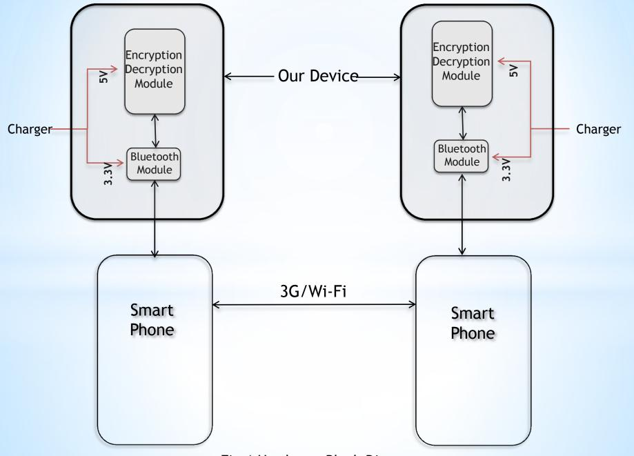
Fig 4:Hardware Block Diagram
